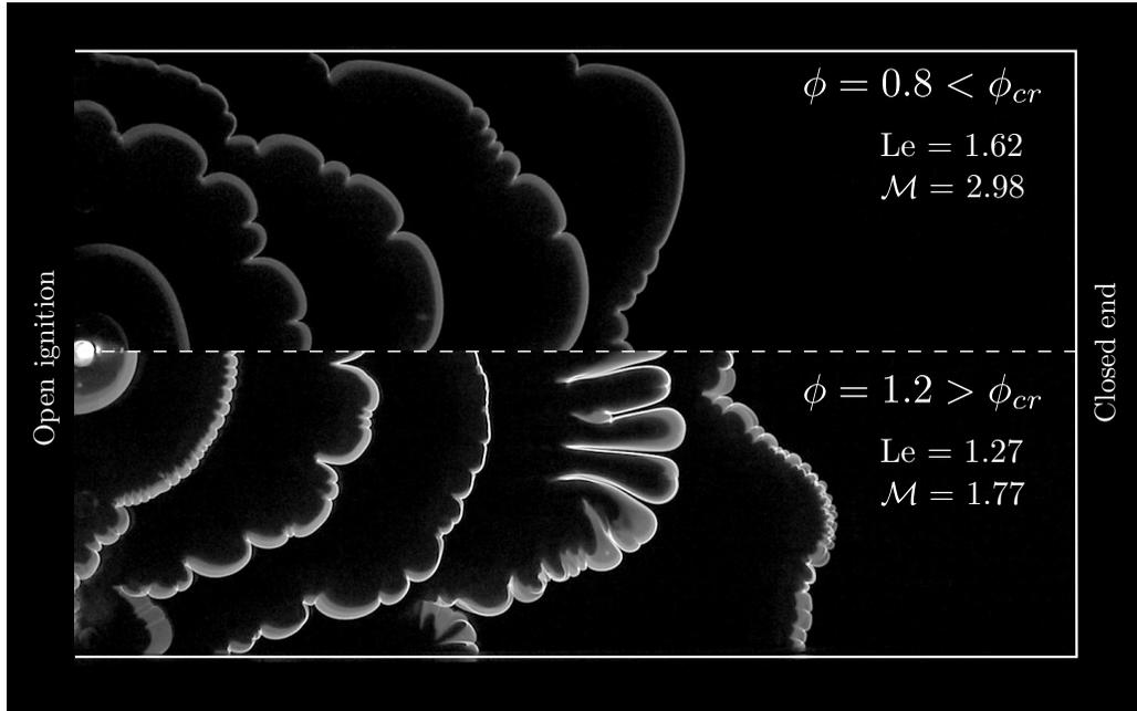
FIG. 1. Top view of premixed propane-air flames propagating in a 900-mm-long, 500-mm-wide, and 10-mm-thick vessel open at the ignition end. <https://doi.org/10.1103/APS.DFD.2018.GFM.V0018>
