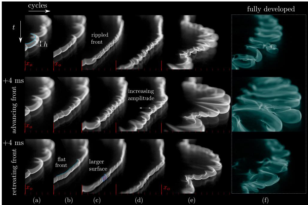
FIG. 2. Side-view detail of the instability transition. Columns (a)–(e) show the reactive front at the beginning, peak, and trough of each cycle. Red vertical lines determine the origin of the picture  $x_o$  (long) and spatial references (short). Column (f) shows fully developed secondary oscillations at a different location. <https://doi.org/10.1103/APS.DFD.2018.GFM.V0018>
