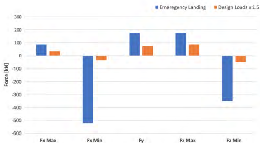
Figure 5.10: Force comparison of design loads and Emergency Landing loads in terms of ultimate loads
