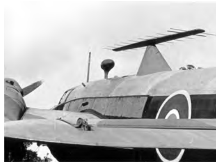
Figure 2.2: Detail view of the Vickers Wellington rotating antenna [24]
