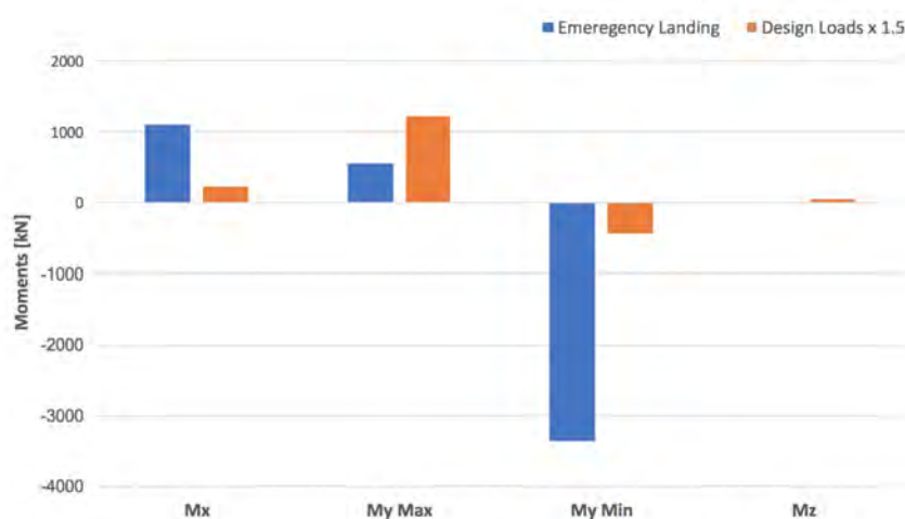
Figure 5.11: Moments comparison of design loads and Emergency Landing loads in terms of ultimate loads
