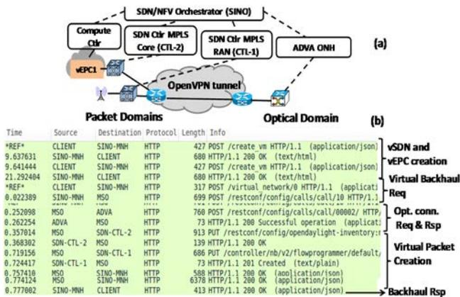
Fig. 7. (a) Setup between CTC SDN/NFV orchestrator and the ADVA ONH.; (b) Capture of the control messages for setting up the VNFs and backhaul.
