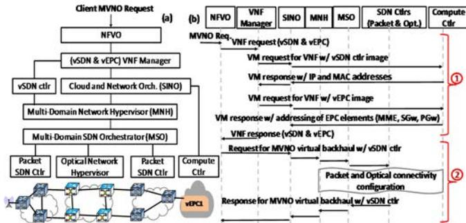
Fig. 6. (a) SDN/NFV orchestration for MVNO backhaul tenants; (b) Workflow creating both backhaul tenant and required VNFs (vEPC and vSDN).
