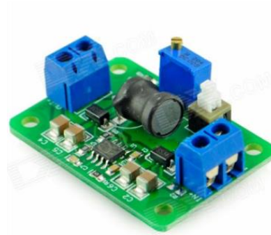
Figura 30: . LM2596 DC-DC Adjustable Step-Down Module. Price: 3,16 US$ [20]
