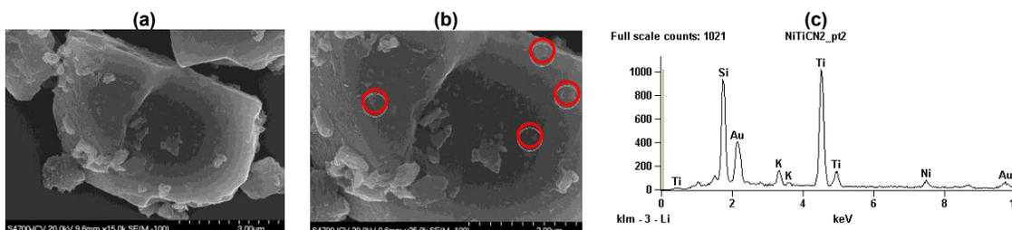
Figure 6 FESEM micrograph of the core-shell Ti(C,N)-Ni (a) y (b) and EDX analysis of the sample (c)
