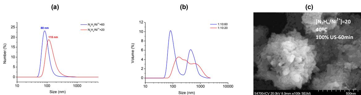
Figure 3 Effect of  $[\text{N}_2\text{H}_4]$  on Dn50 (a) and Dv50 (b) and FESEM micrograph of the sample obtained with  $[\text{N}_2\text{H}_4/\text{Ni}^{2+}] = 20$  (c)
