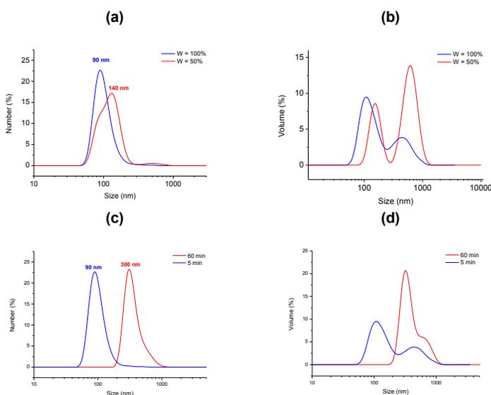
Figure 5 Effect of the ultrasonic power and time respectively on Dn50 (a and c) and Dv50 (b and d)
