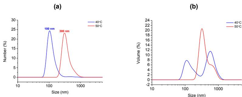
Figure 4 Effect of the temperature on Dn50 (a) and Dv50(b)
