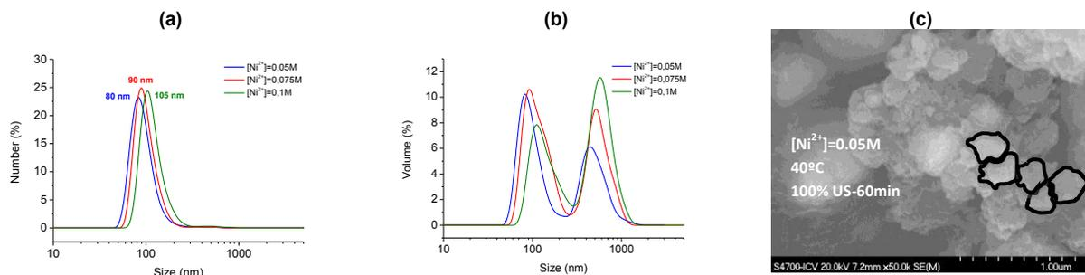
Figure 2 Effect of initial  $[\text{Ni}^{2+}]$  on Dn50 (a) and Dv50 (b) and FESEM micrograph of the sample obtained with  $[\text{Ni}^{2+}] = 0.05\text{M}$  (c)
