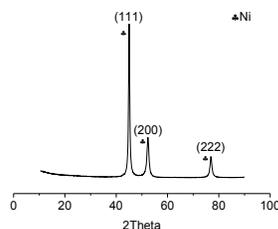
Figure 1 X-Ray Diffraction pattern of nickel
