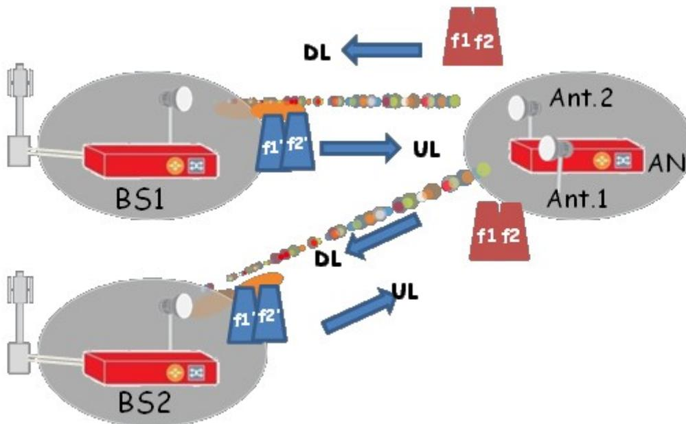
Figure 3. Full frequency reuse due to enough antenna separation
