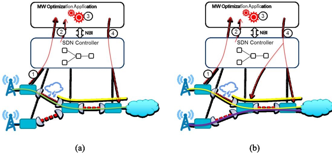
Figure 1. Selective traffic shaping (a) and re-routing (b).
