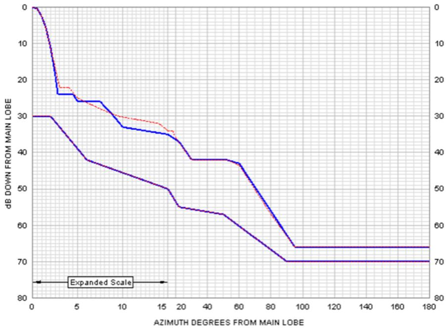
Figure 6: 2ft antenna radiation pattern at 18 Ghz.
