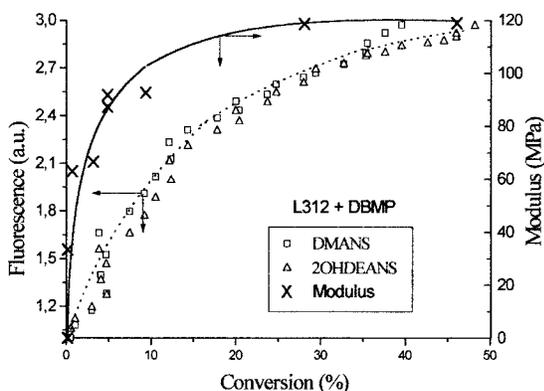
**Figure 7.** Plot of the fluorescence changes versus the conversion during the UV curing of L312 with DBMP. The fluorescent probes were DMANS and 2OHDEANS. On the right axis, the shear modulus of the adhesives formulations as a function of conversion is plotted.  $I_0 = 1.84 \text{ mW} \cdot \text{cm}^{-2}$ .
