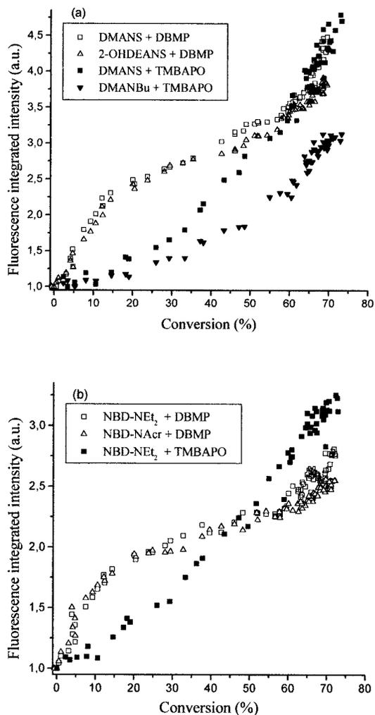
**Figure 5.** Plots of the fluorescence versus the conversion of the UV curing of the adhesive L312 with DBMP and TMBAPO as photoinitiators. The fluorescent probes were (a) DMANS, DMANBu, and 2OHDEANS and (b) NBD derivatives.  $I_0 = 1.84 \text{ mW} \cdot \text{cm}^{-2}$ .
