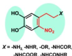
Mussel glue: Bioinspired underwater chemical bonding with the possibility of phototriggered debonding is reported. A four-arm star-poly(ethyleneglycol) end-functionalized by nitrodopamine was synthesized. The nitrodopamine offered the reactivity of catechol and the chemistry of the photocleavable *o*-nitrophenyl ethyl group (see picture).
