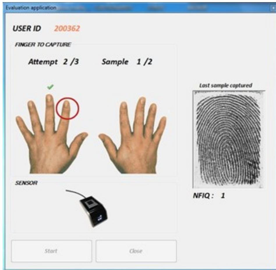
Figure 48. App Interface of the enrolment. There are several elements intended to help the user and the evaluator (finger to present, device, attempt, sample, fingerprint quality (NFIQ), image and user ID)
