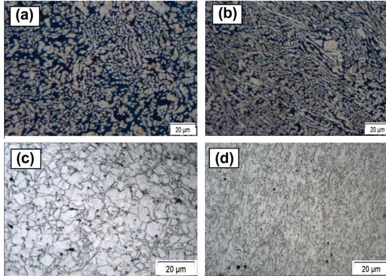
**Fig. 2.** Cross sectional views of the microstructure of the corrugated bars: (a) core of CW 2205 (b) outer region of CW 2205 (c) core of the HW 316L (d) outer region of the HW 316L.
