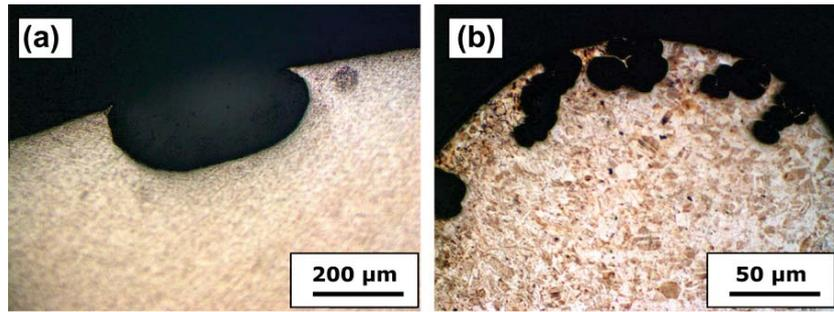
**Fig. 12.** Cross-sectional views of the morphology of the pits in specimens manufactured from the cores of the bars after polarization in solutions with chlorides: (a) HW 304L; (b) CW 304L.
