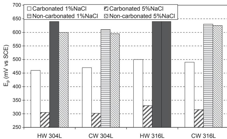
Fig. 10.  $E_p$  values obtained for the core of the bars in carbonated and non-carbonated solutions with chlorides. Black bars represent systems where water decomposition conditions are reached, and pitting does not take place.
