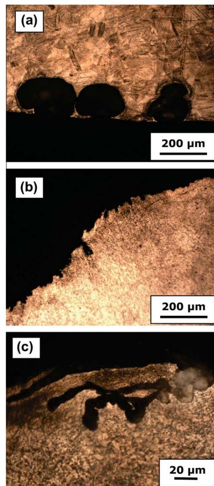
Fig. 11. Cross-sectional views of the morphology of the pits in corrugated surfaces after polarization in solutions with chlorides: (a) CW 304L; (b) HW 304L (predominant way of attack); (c) HW 304L (detail of the most strained region).
