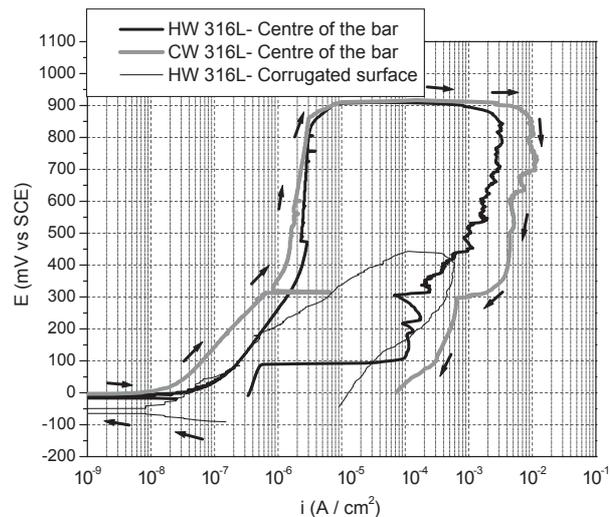
**Fig. 9.** Polarization curves for the cores of HW and CW 316L bars in carbonated solution with 1% NaCl. Curve corresponding to the corrugated surface of one of the materials in that media is included for comparison.
