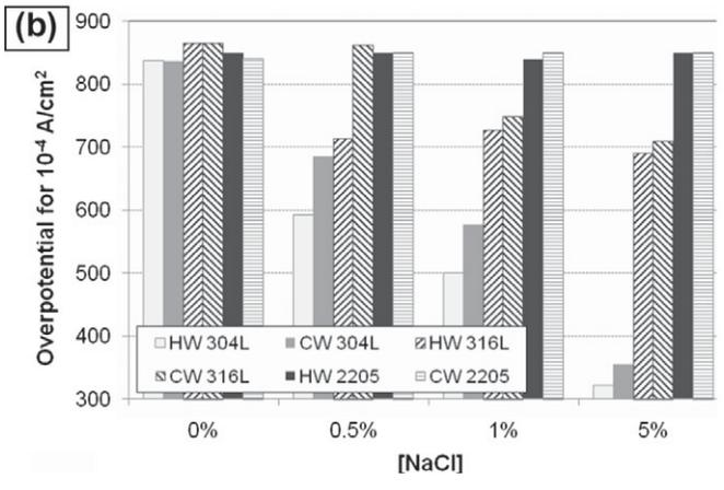
Fig. 7. Anodic overpotentials for the studied corrugated stainless steels in non-carbonated solutions: (a) for reaching  $5 \times 10^{-6} \text{ A/cm}^2$ ; (b) for reaching  $10^{-4} \text{ A/cm}^2$ .
