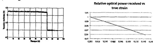
a) Voltage measured at reception vs time b) Relative optical power vs true strain
