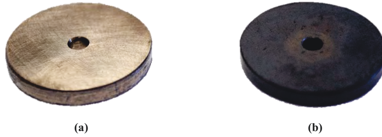
Figure 5.18. Piece of Inconel 718 (a) as-rolled and –received (b) as-received and oxidized for 2hours at 650°C.
