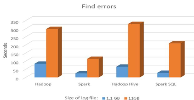
Figure 13: Execution times of find errors programs and SQL-type queries.
