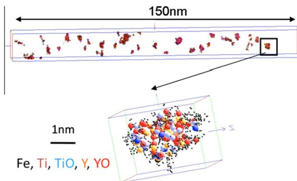
**Fig. 4.** Atom probe tomography analysis of the chemical composition of nano-clusters evidenced in an ODS RAF steel powder produced by reactive ball milling between Fe–Cr–W–Ti powder particles, YFe<sub>3</sub> particles and Fe<sub>2</sub>O<sub>3</sub> particles [11].
