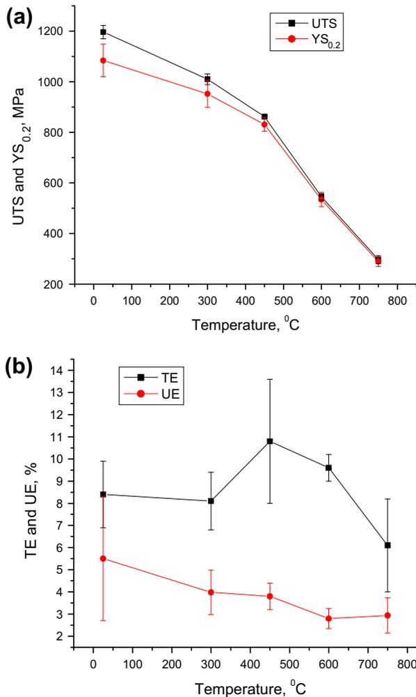
**Fig. 3.** Tensile properties versus test temperature of a Fe-14Cr-2W-0.3Ti-0.3Y<sub>2</sub>O<sub>3</sub> ODS RAF steel prepared by mechanically alloying pre-alloyed powder particles with Y<sub>2</sub>O<sub>3</sub> particles in an attritor, HIPping, hot rolling and heat treatment at 850 °C: (a) yield strength (YS<sub>0.2</sub>) and uniform tensile strength (UTS), (b) uniform elongation (UE) and total elongation (TE).
