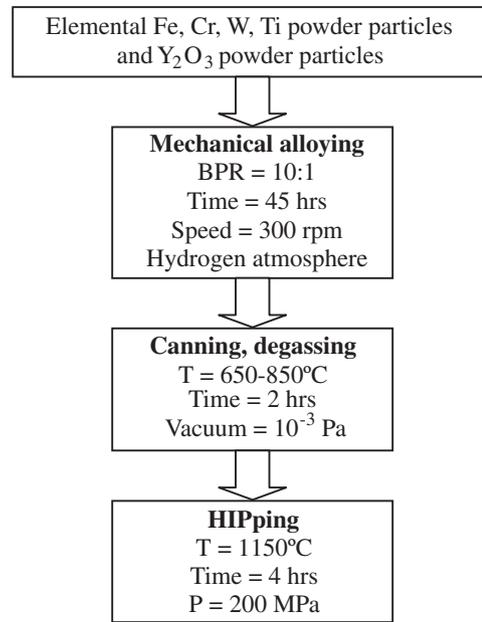
Fig. 2. Optimal processing conditions for a Fe-14Cr-2W-0.3Ti-0.3Y<sub>2</sub>O<sub>3</sub> ODS RAF steel prepared by mechanically alloying elemental powder particles with Y<sub>2</sub>O<sub>3</sub> particles in a planetary ball mill and HIPping.
