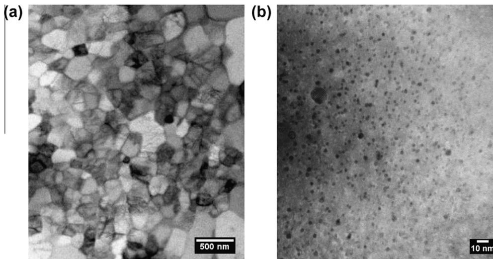
Fig. 1. Transmission electron microscopy images of the microstructure of a Fe-14Cr-2W-0.3Ti-0.3Y<sub>2</sub>O<sub>3</sub> ODS RAF steel prepared by mechanically alloying elemental powder particles with Y<sub>2</sub>O<sub>3</sub> particles in a planetary ball mill and HIPping: (a) general view and (b) high magnification image of 5-6 nm nano-clusters.
