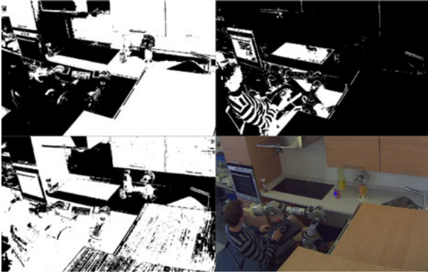
Fig. 16. Color segmentation and object centroid on kitchen IP camera image.
