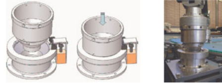
Fig. 5. ASIBOT docking mechanism: tip inserted and locked into a DS.
