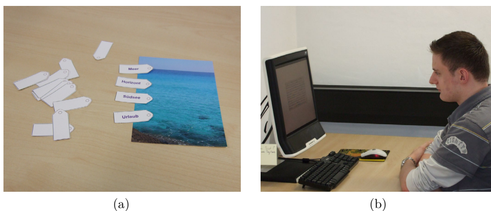
Figure 5.4 — a) Paper demonstrator to explain tagging and tag clouds, b) Presentation of the tag clouds on a 17" TFT monitor with embedded eye tracking system.
