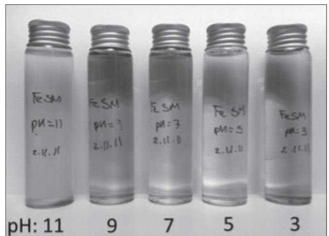
Figure 2. Picture of wastewater showing the Fe oxidation vs. pH.
