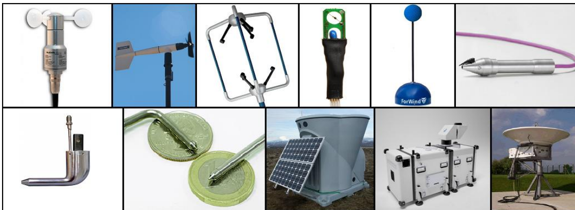
Figure 2: Common sensors for atmospheric wind speed measurement. From left to right and from top to bottom: Cup anemometer, propeller anemometer, sonic anemometer, hot-wire anemometer, sphere anemometer, laser-cantilever anemometer, pitot tube, multi-hole probe, sodar, lidar and radar
