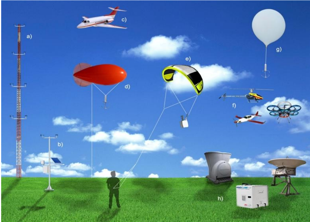
Figure 1: Platforms for wind measurement characterization. a) Meteorological mast, b) Weather station, c) MAV, d) Tethered balloon, e) Kite, f) UAVs, g) Radiosonde, h) Sodar / lidar / radar
