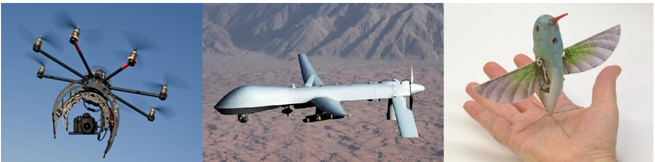
Figure 4: Examples of Unmanned Aerial Vehicles. From left to right: Hexacopter, MALE RQ-1 Predator and NAV "Nano Hummingbird" (flapping-wing UAV configuration)
