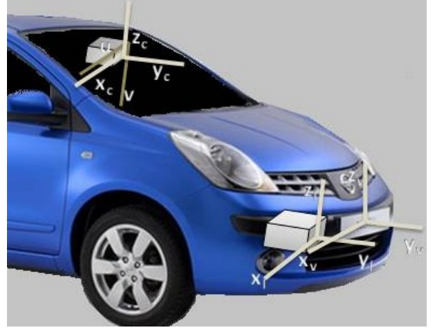
Figure 4. Different coordinate systems ( x_c, y_c, z_c ) are camera coordinate system, ( x_l, y_l, z_l ) is the laser coordinate system, and ( x_v, y_v, z_v ) is the coordinate system of the vehicle. Coordinates ( u, v ) are the image coordinates.
