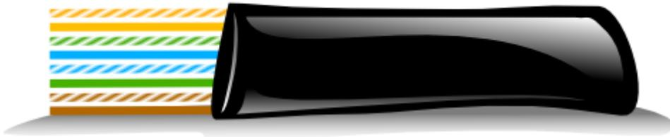
Figura 3. 25 Cable RJ45[7] recortado
