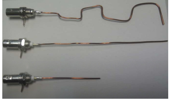
Figure 3. Zig-zag, 10 cm monopole and 5 cm antennas
