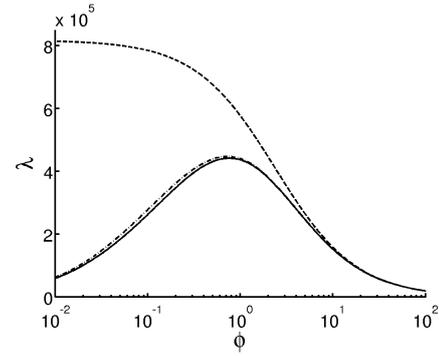
Figure 5: The variation with composition of  $\lambda$  at  $T = 1200$  K and  $p = 1$  atm (solid curve) together with the approximate solutions  $\lambda = 2k_{1f}C_{O_2}$  (dashed curve) and  $\lambda = 2k_{1f}C_{O_2}\Lambda$  (dot-dashed curve).
