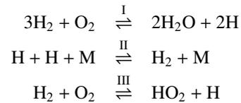
with global rates given in (2). Note that, although the reduced chemistry can be expressed in terms of different alternative sets of overall reactions, the resulting formulations are all equivalent. The one selected here is written in an intuitive form that serves to identify the main chemical processes involved in hydrogen combustion, i.e., it includes a branching reaction I, a recombination reaction II and an initiation reaction III.
