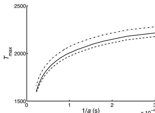
Figure 2: The variation with strain rate of the maximum temperature in a hydrogen-air planar counterflow at atmospheric pressure with feed-stream temperatures  $T = 300$  K as obtained with the detailed 21-step chemistry (solid curves), with the short 12-step chemistry (dashed curves) and with the 3-step reduced mechanism (dot-dashed curves).
