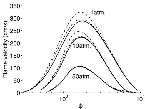
Figure 1: The variation with equivalence ratio of the laminar burning rate of hydrogen-air planar deflagrations with initial temperature  $T_u = 300$  K and three different pressures as obtained with the detailed 21-step chemistry (solid curves), with the short 12-step chemistry (dashed curves) and with the 3-step reduced mechanism (dot-dashed curves).
