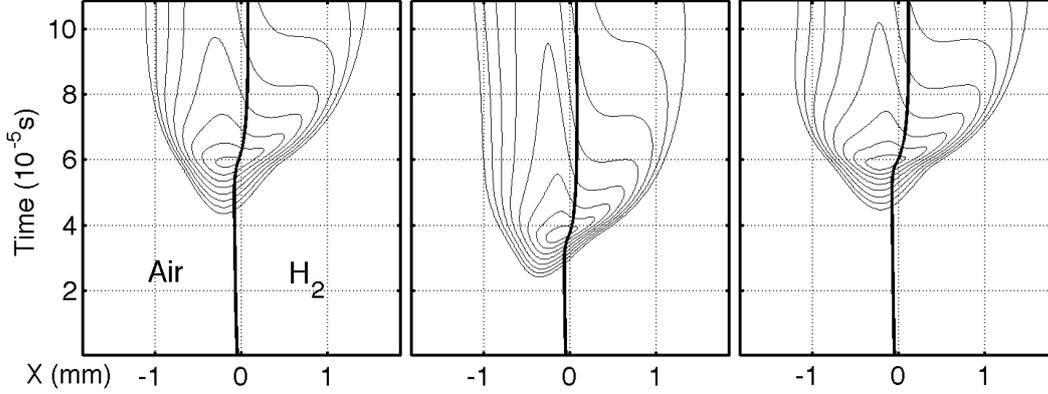
Figure 4: Isocontours of heat-release rate corresponding to  $2^n \times 6.14 \times 10^7 J.m^{-3}.s^{-1}$  for  $n = 0$  up to  $n = 7$  in the transient one-dimensional  $H_2$ /air mixing layer at atmospheric pressure and initial temperature 1200K as obtained with the 21-step chemistry (left plot), with the 3-step reduced chemistry (centered plot) and with the modified 3-step reduced chemistry (right plot) ; the black line indicates the location where the mixture is stoichiometric.
