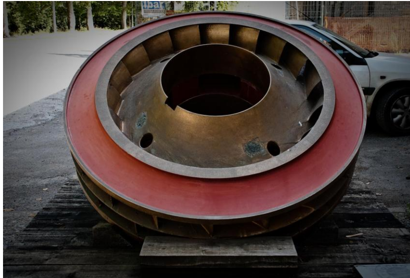
Bronze wheel from Seira hydroelectric plant.(3)
