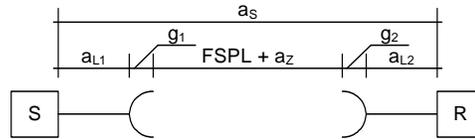
Figure 2. Loss Parameters within a System as shown in Equation 4
