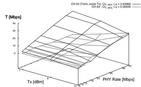
Figure 21. Throughput Measurement for TxTx Case, Channel Separation of 3 and with NoAck Policy Enabled
