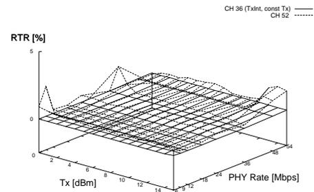
Figure 13. Retransmission Rate for Channel Separation of 4 and Antenna Separation of 20 cm
