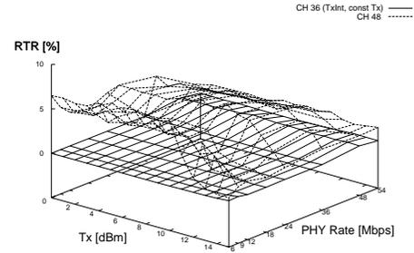
Figure 11. Retransmission Rate for Channel Separation of 3 and Antenna Separation of 20 cm
