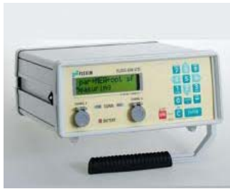
Figure B.2 Ultrasonic flow meter Flexim-Fluxus AMD 6725
