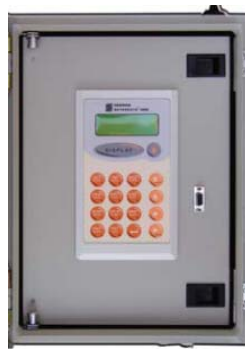
Figure B.1 Weather data acquisition system: Meteodata-3008CM
