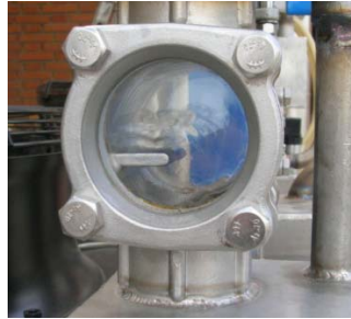
Figure 3.2 Detail of the vapor flow viewer at the outlet of each generator
