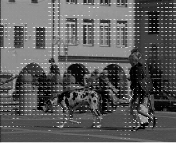
Figure 3. Motion vector map calculated by HME.
