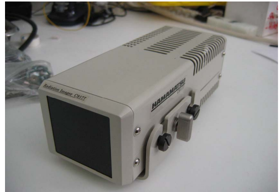
Figure 1. Front view of the Hamamatsu C9177 radiation imager. The system also includes a supply module, a connector box and a PCI interface. The approximate weight of the detector head is 2 Kg.
