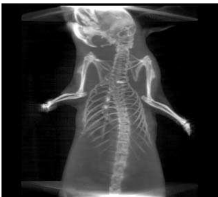
Figure 1. Brightest point volume rendering from 3-D SART reconstructed volume of 280 \times 280 \times 280 voxels. Note the cone-beam artifact in the upper and lower slices due to the 180 degrees projection data restriction.
