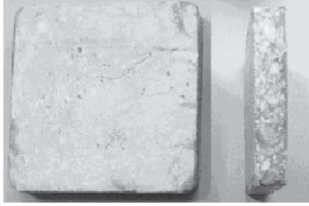
Fig. 3. Tile of vinyl ester resin and alumina particles. Front view (left) and cross-section (right).
