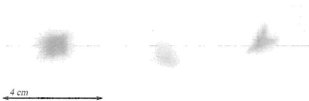
Fig. 20. Impact point of 5 J impacted specimens ( 10 \times 10 cm), backlight picture.
