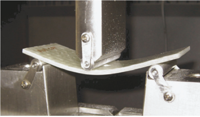
Fig. 4. Experimental three-points bending test configuration.
