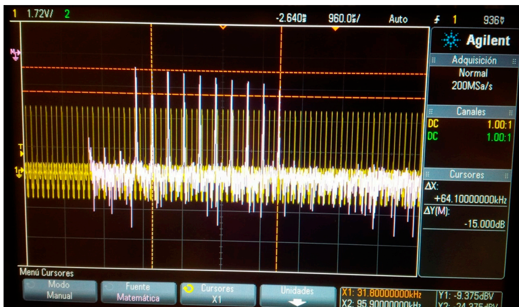
Figure 6. Synthetic noise for EN 50065 limits with frequency peaks every 8 kHz.
