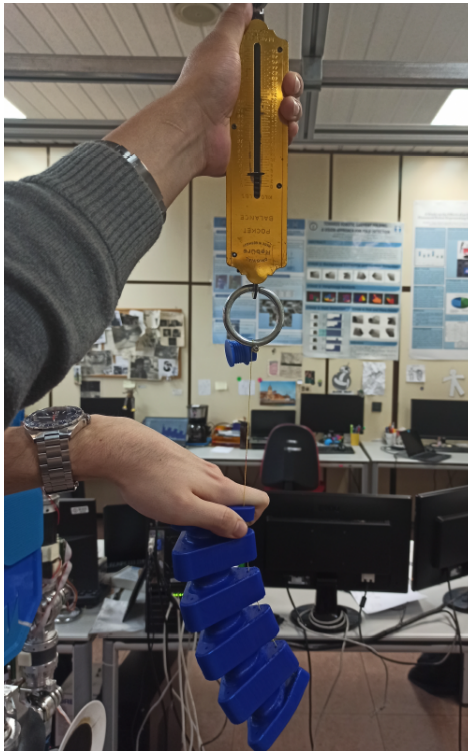
Figure 3.36: Experimental measurement to obtain a hypothetical value of the necessary linear forces.
