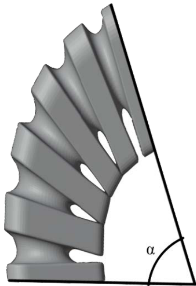
(a) Flexion in configuration 1 has the lowest maximum bending angle.
