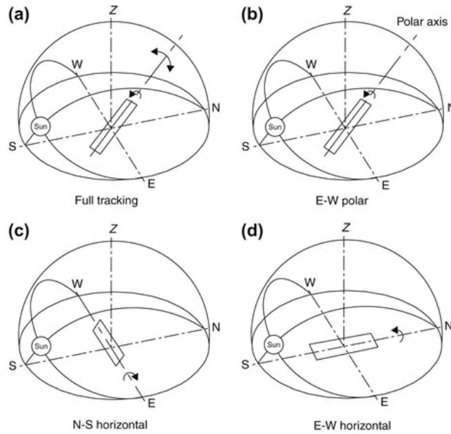
FIGURE 15 Collector geometry for various modes of tracking [13]
