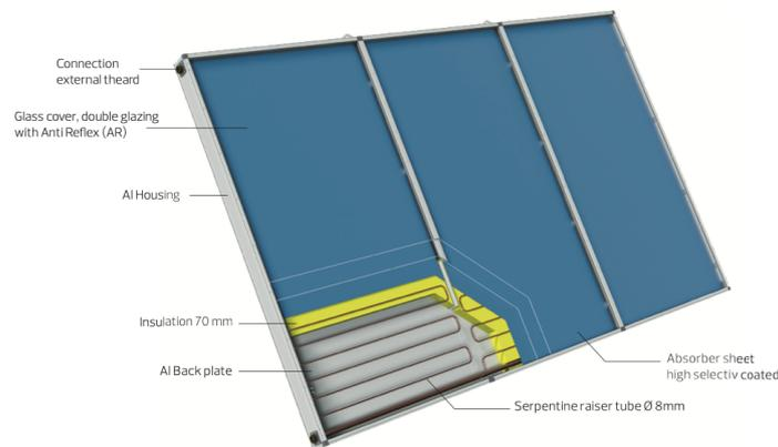
FIGURE 46 Schematic of the solar flat plate collector [40]
