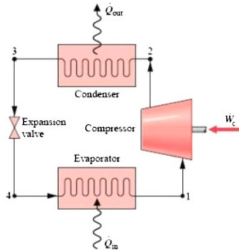
FIGURE 33 Vapor compression system [33].
