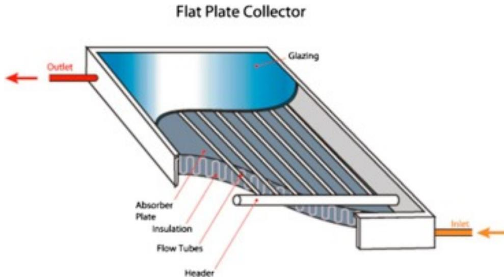
FIGURE 18 Schematic of a typical flat collector [19]
