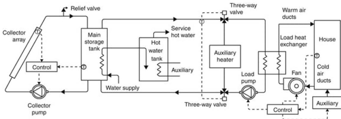
FIGURE 30 Schematic diagram of a solar space-heating and hot water system. [30]
