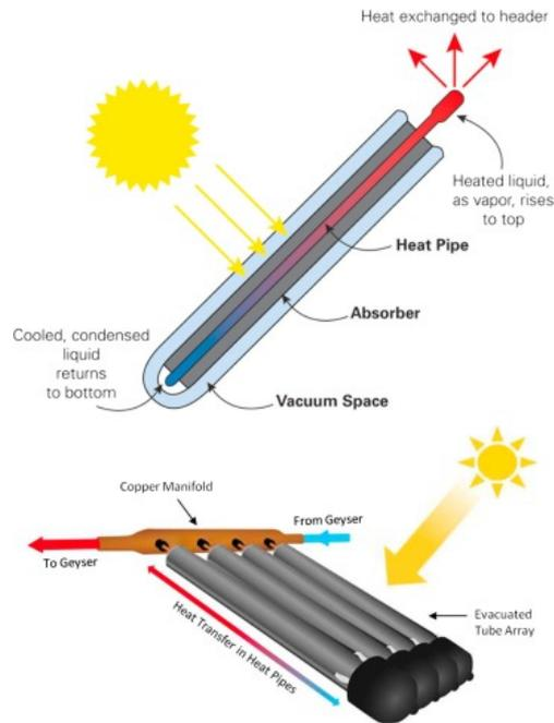
FIGURE 19 Schematic diagram and operating principle of an ETC [19]
