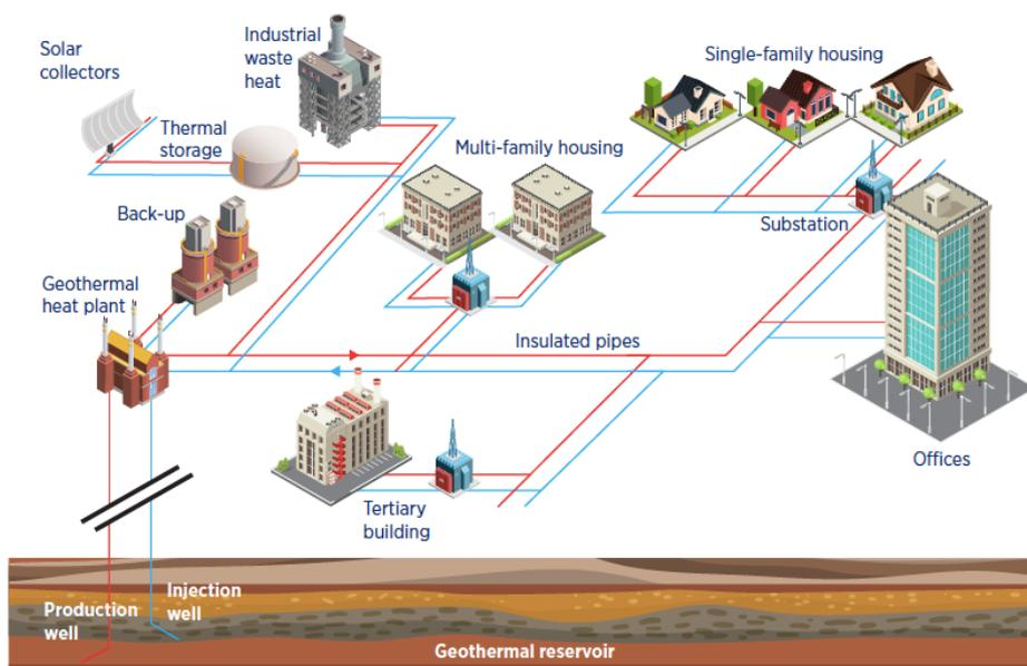
FIGURE 11 Schematic diagram of a district heating system using multiple energy sources [2]
