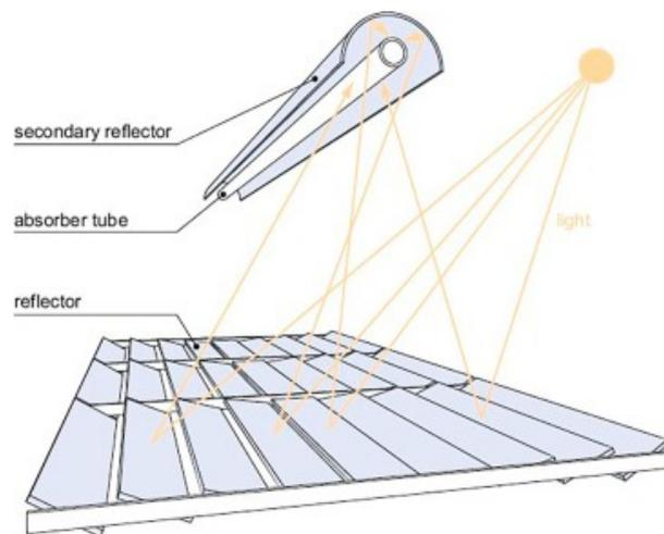
FIGURE 23 Schematic representation of a Linear Fresnel collector [19]
