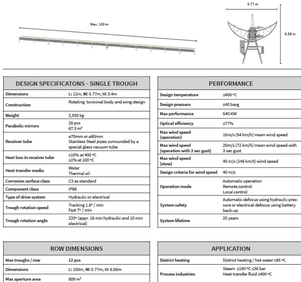
FIGURE 48 Technical sheet parabolic trough collector[41]
