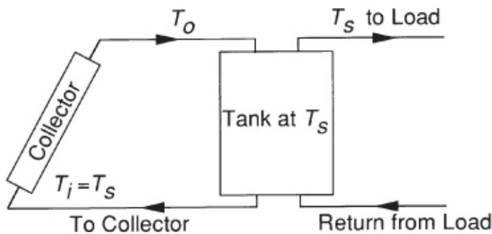
FIGURE 25 A typical system using water tank storage, with water circulation through collector to add energy and through the load to remove energy. [25]
