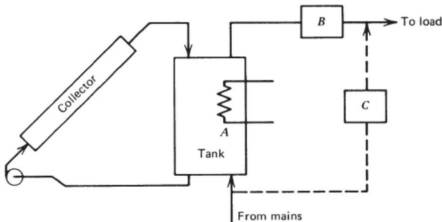
Figure 24 Schematic of alternative location for auxiliary energy supply to a one-tank forced-circulation solar water heater: A, in tank; B, in line to load; C, in a bypass around tank. [24]
