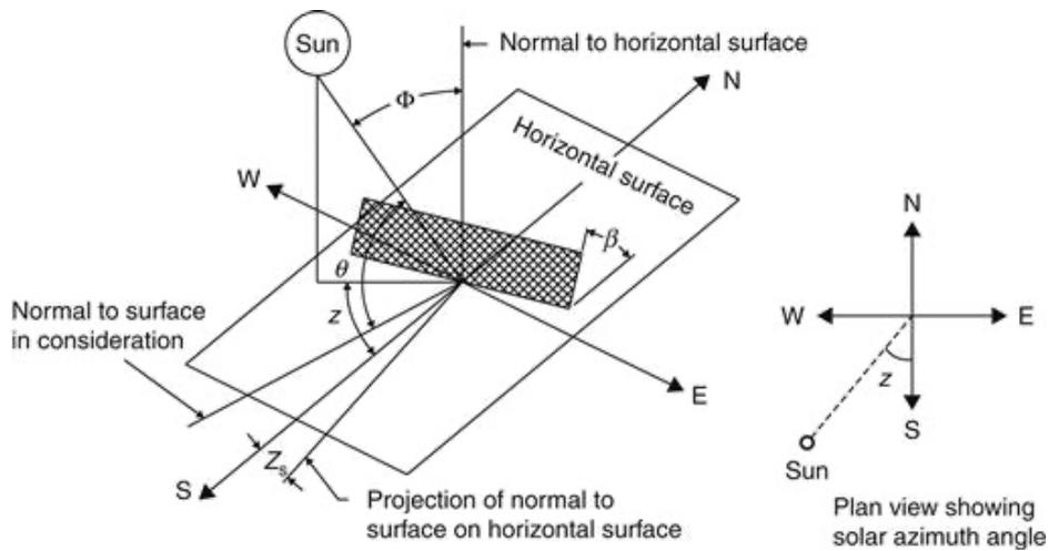
FIGURE 14 Solar angles diagram[13]
