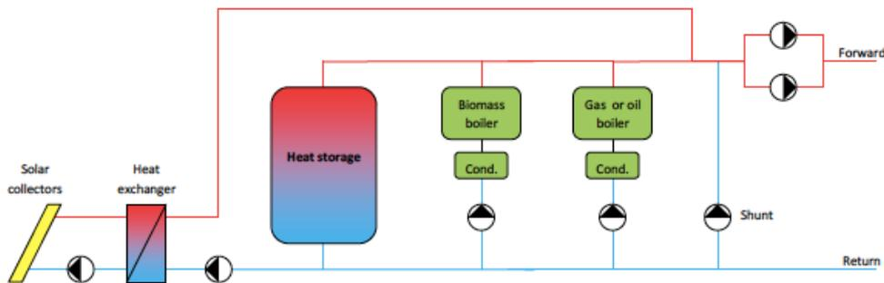
FIGURE 61 Example of combined solar and biomass in parallel configuration[44]
