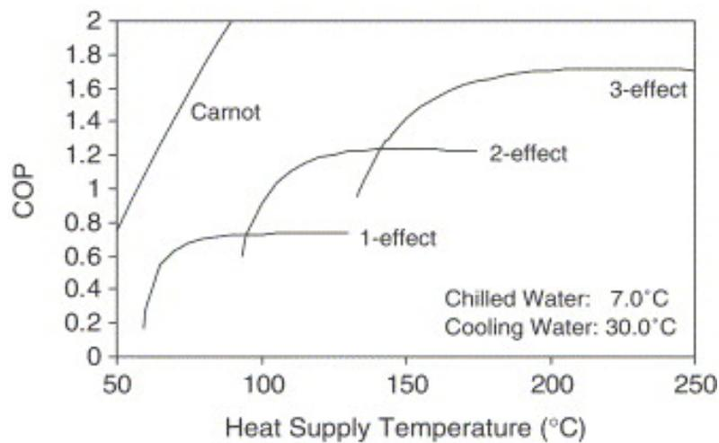
FIGURE 37 Coefficient of Performance (COP) as a function of solar heat supply temperature for single-, double- and triple-effect LiBr–water absorption chillers.[37]
