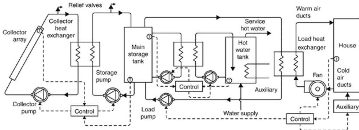
FIGURE 31 Detailed schematic diagram of a solar space-heating and hot water system with antifreeze solution [30].
