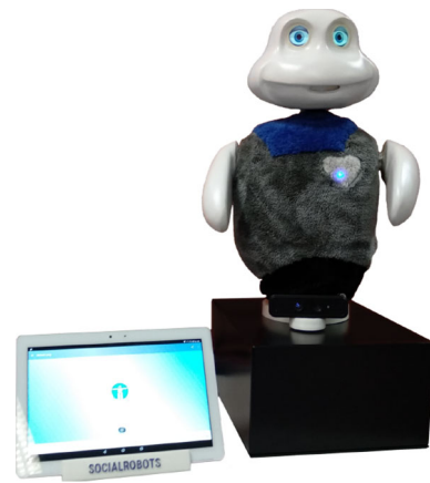
Fig. 4 The Mini social robot, which is used as the platform where our affective model has been implemented to generate and express affective states
