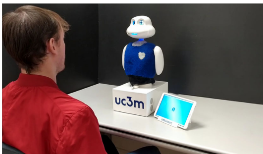
Fig. 6 Case study where the Mini social robot interacts by playing a quiz game. The robot's affective state is modulated depending on the dynamics of the interactions and expressed to inform the user how it feels
