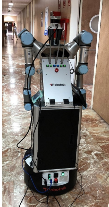
Figure 1.1: ADAM: Mobile manipulator platform developed in the Robotics Lab.
