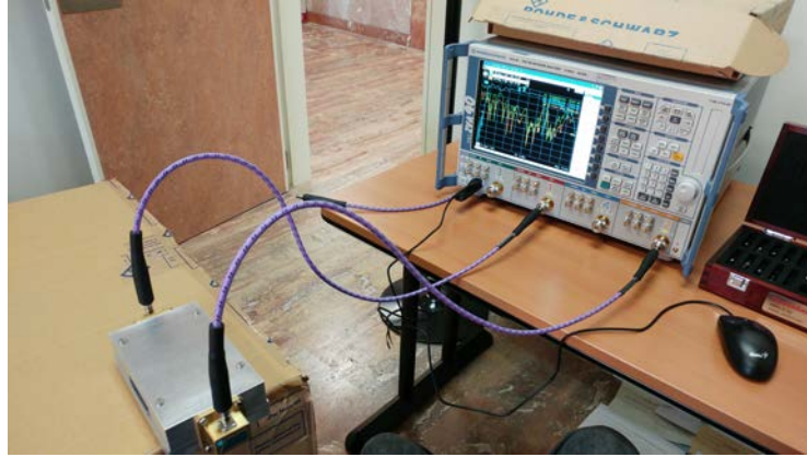
Figure 5.19: Prototype #1 (B2B Groove Gap Waveguide to Microstrip transition without amplification): Measurement process with VNA ZVA40.
