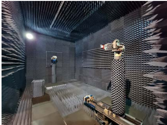
(c) Installed antenna on the positioner (panoramic view).
