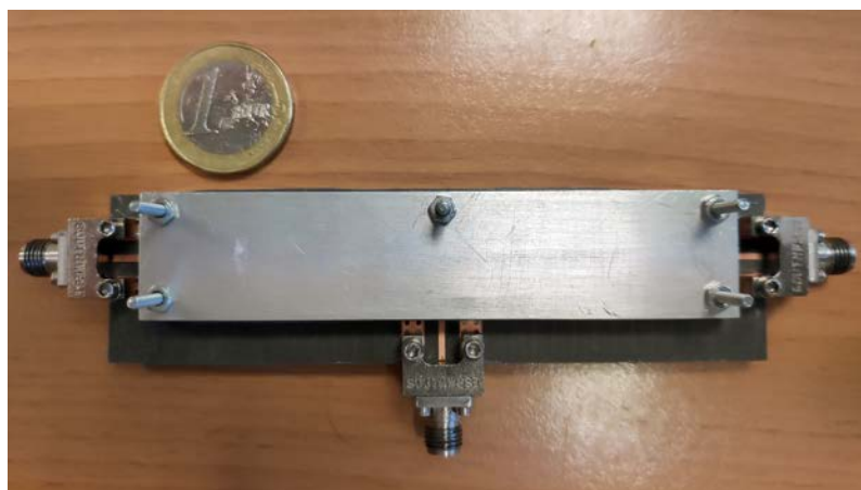
(c) Top of assembled diplexer with transition and connectors.
