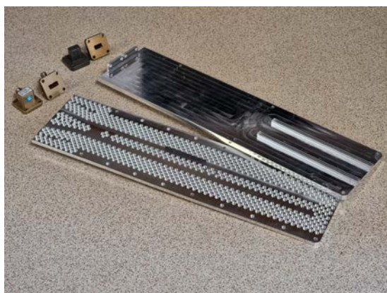
(a) Top and bottom lids. WR34 transitions and Matched Loads 50 \Omega .
