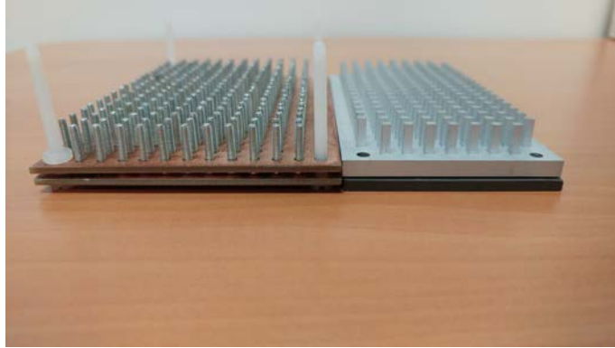
Figure 1.16: Low cost bed of nails with screws vs. new bed of nails machined with metal pins.
