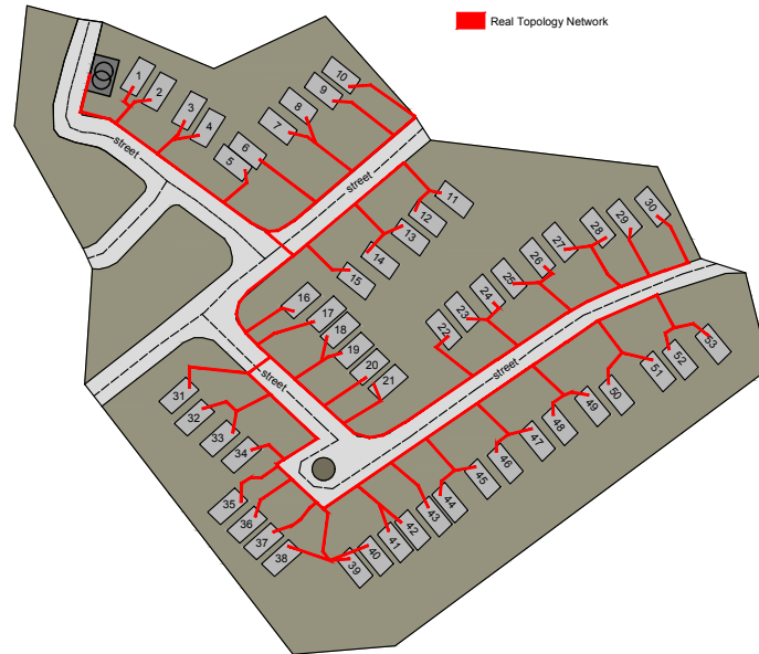
Figure 5.4: European low-voltage test feeder topology representation
