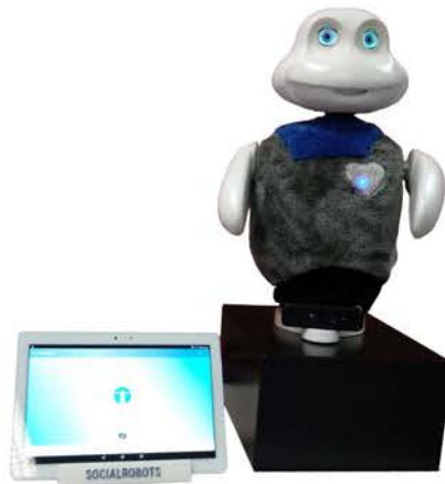
Figure 5.1: Front view of the social robot Mini and the tablet device attached to it.
