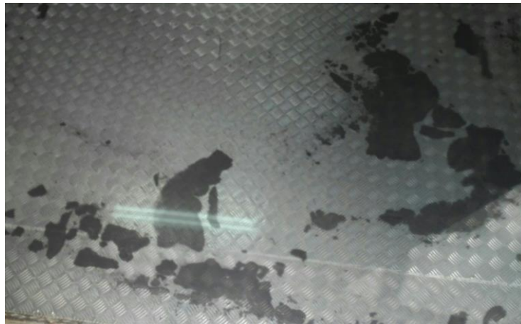
Figure 2. Residues deposited on the floor of the camera after test.
