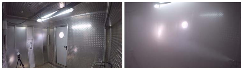
Figure 1. Fog Dynamics Laboratory. Test room before and after the release of the cleaning fog.
