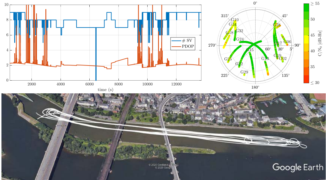
Figure 6.10: On the upper left, the number of tracked satellites and associated PDOP. On the upper right, the skyplot of the scenario, with the colorbar indicating the C/N_0 . In the bottom, the trajectory followed by the tracked vessel during bridge passing, estimated using laser technology.
