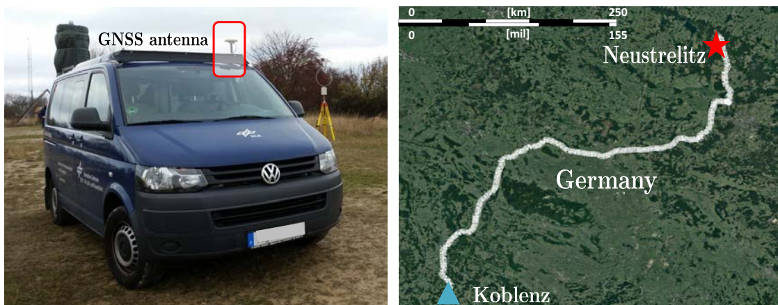
Figure 5.8: Experimental setup for the evaluation of robust code-based positioning under real conditions. On the left, the tracked vehicle and a highlight for the position of the antenna. On the right, the route traversed during the data collection, with starting and finish points in the cities of Koblenz and Neustrelitz (Germany), respectively.
