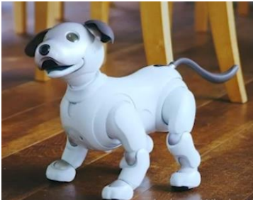
Figure 2.18 Aibo robot ( aibo - Specification , 2019).
