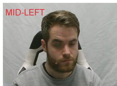
Figure 6.7. Eye gaze system results: the pupil position (green circle), calibration point (red circle), and gaze area estimation (red text).
