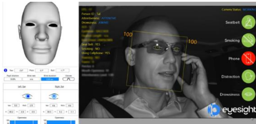
Figure 2.3. Driver Sense software-based DMS of Cippa Vision Ltd 1 .
