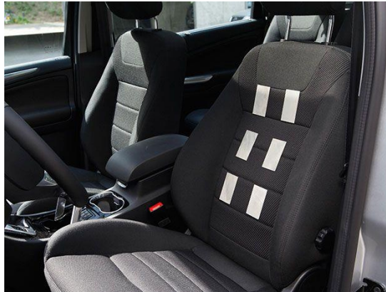
Figure 2.5. Driver's seat prototype that integrates an ECG sensor designed by Ford 2
