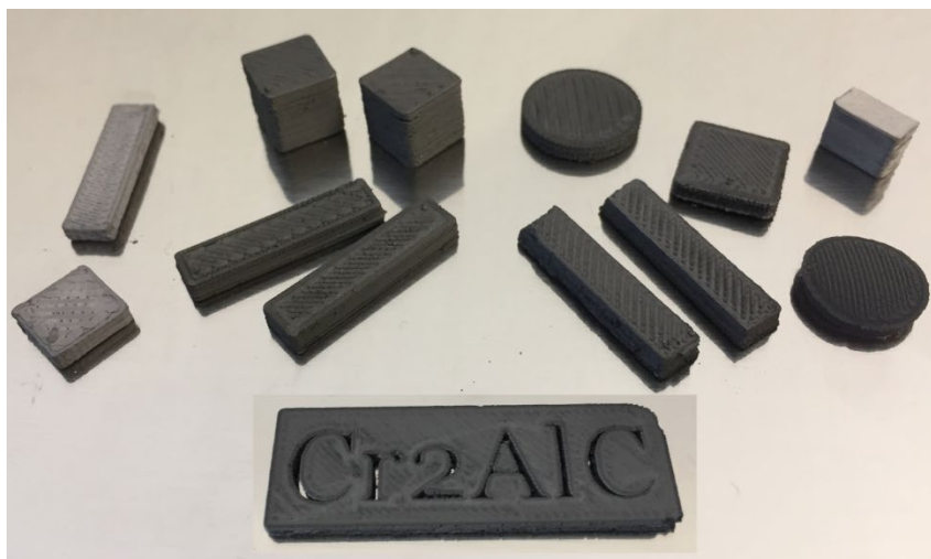
Figure 25. Image of some of the geometries printed for the optimisation process during this work.
