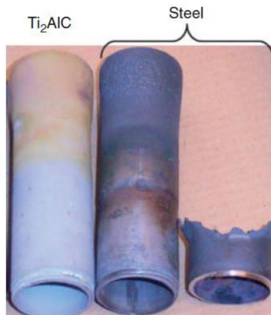
Figure 9. Gas burner nozzles of Ti_2AlC and steels tested in service at 1400 °C [8].
