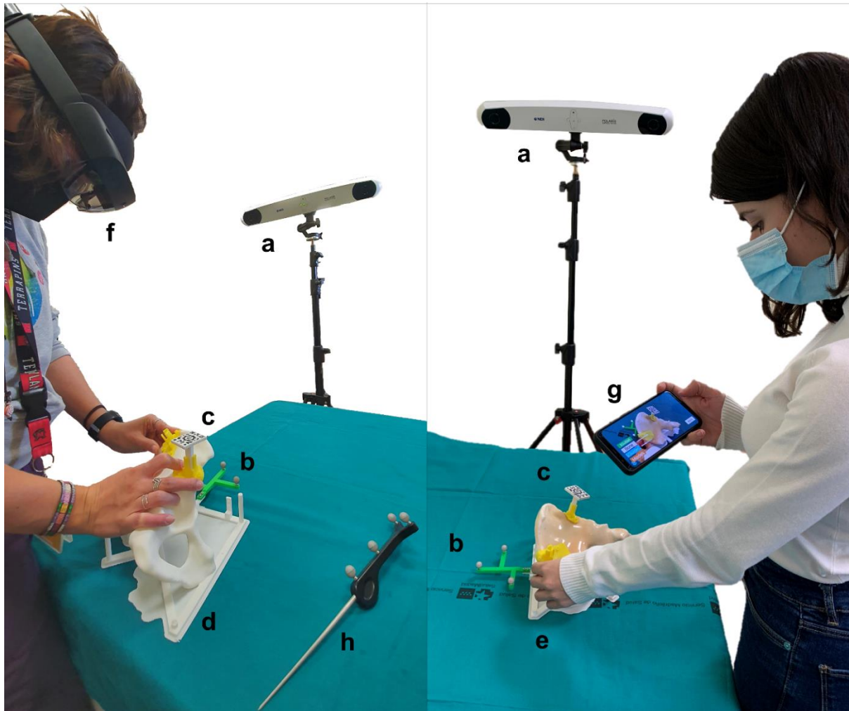
Figure 5.3. Setup for the assessment using (left) the HoloLens 2 and (right) the smartphone. The setups include the following elements: (a) optical tracker, (b) reference frame, (c) AR marker placed in PSI, (d) conventional, and (e) realistic phantom versions, (f) HoloLens 2, (g) smartphone, and (h) pointer.
