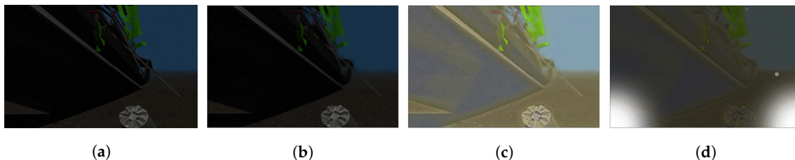
Figure 5. Example of each processing step on an input image. (a) Original image from the UUV Simulator. (b) Forward-scattered image. (c) Result of applying style transfer to the forward-scattered image. (d) Addition of two light sources on each of the bottom corners.
