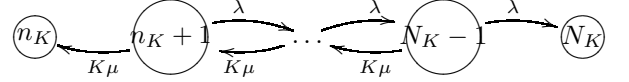
Fig. 3. CTMC for Stage K : K active APs and no AP powering on
