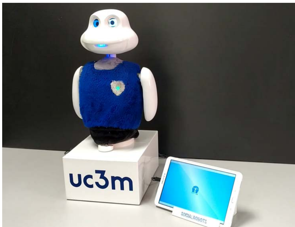
Figure 2.2: Mini, a social robot designed for assisting older adults suffering from cognitive impairment.
