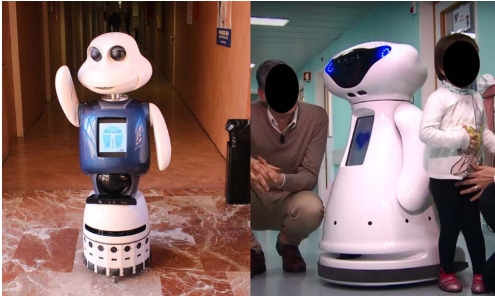
Figure 2.1: Maggie, a social robot designed as a research platform (left), and Mbot (right), a robot for entertaining children in a hospital (source: [2]).
