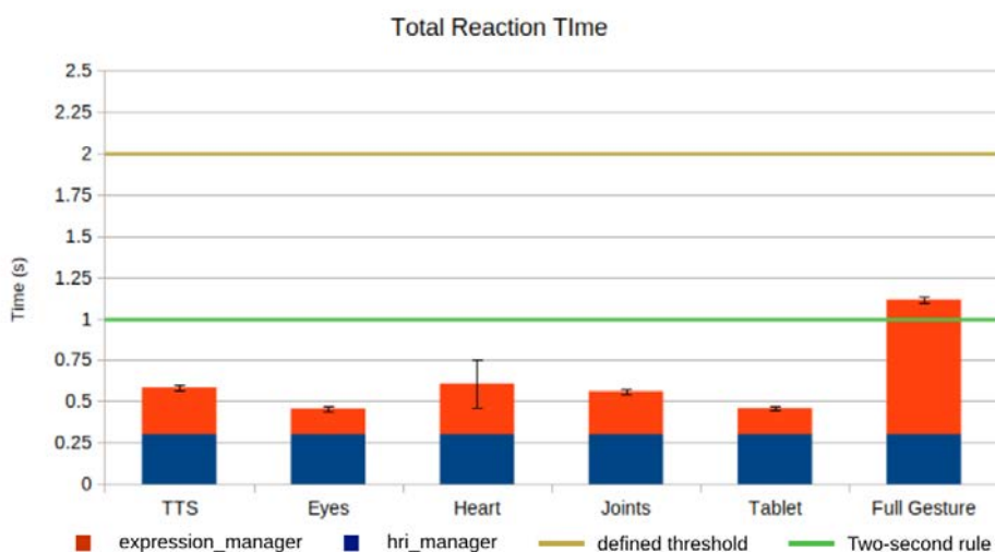
Figure 4.11: Reaction time for the combination of the HRI Manager and the Expression Manager. The bars represent the average value, the whiskers represent the standard deviation, and the horizontal bars represent the two thresholds defined for interactions between the robot and the human.
