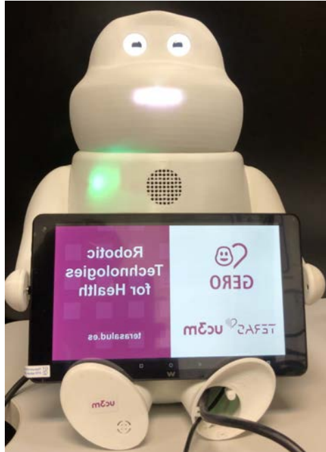
Figure 2.3: Gero, a low-cost social robot designed for assisting older adults suffering from mild cognitive impairment.
