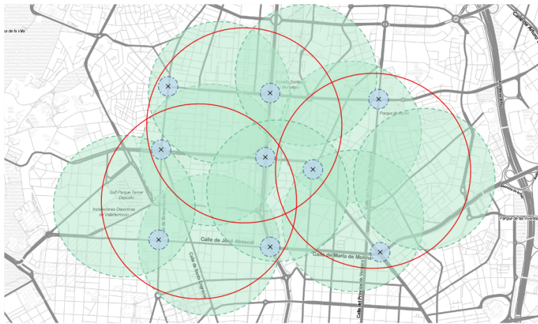
Figure 5.8: Road topology used in the large-scale scenario. The nine crossings correspond to endpoints; red, green, and blue circles represent the coverage areas of macro-, micro- and pico-cells, respectively.
