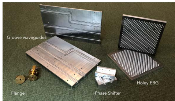
Figure 20. Manufactured prototypes using glide-symmetrical holey structures. Further details can be found in [154, 167–169].
